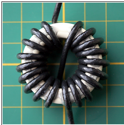
Traditional low-capacitance construction with split winding.
